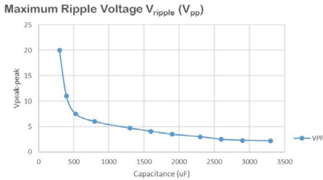
Figure 8: Example - Capacitance values versus ripple voltage [Source: Rambow-Technology]
