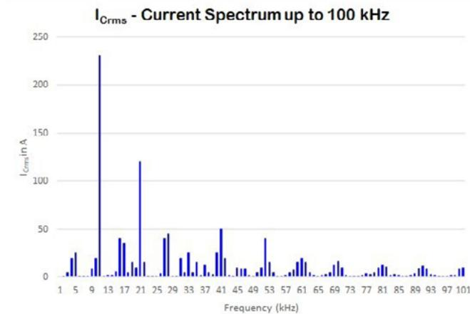
Figure 9: Amplitude of I<sub>Crms</sub> gaining losses up to 100 kHz [Source: Rambow-Technology]
