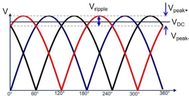
Figure 6: Simplified DC-link voltage switching ripple ( $V_r$ )
