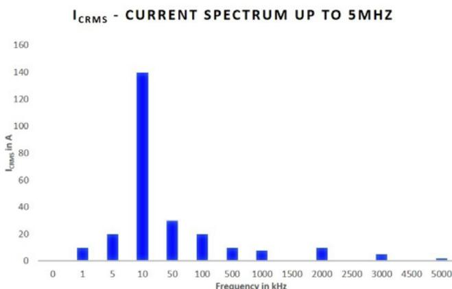
Figure 10: Amplitude of I<sub>Crms</sub> gaining losses up to 5 MHz [Source: Rambow-Technology]
