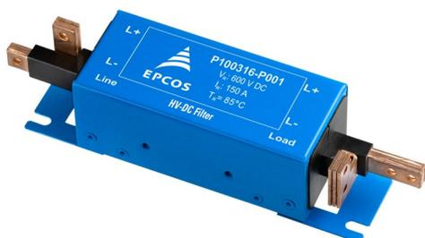
Figure 4: EPCOS high-voltage DC filters for automotive inverters. The connections of Version P001 are formed in such a way that they can be connected directly to the EPCOS DC-link capacitor. Apart from the space-saving design, they also offer electrical advantages such as low inductance and contact resistances.
